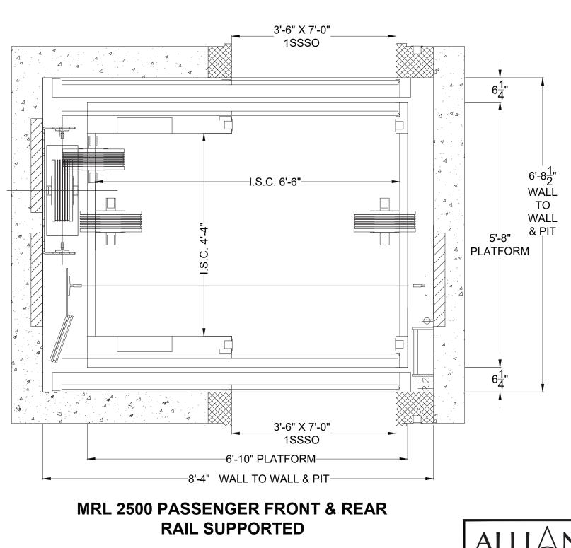
DIMENSIONS SHOWN ARE FOR SEISMIC ZONE 0, ADD 2" ON EACH SIDE **FOR ZONE 2 OR GREATER**
